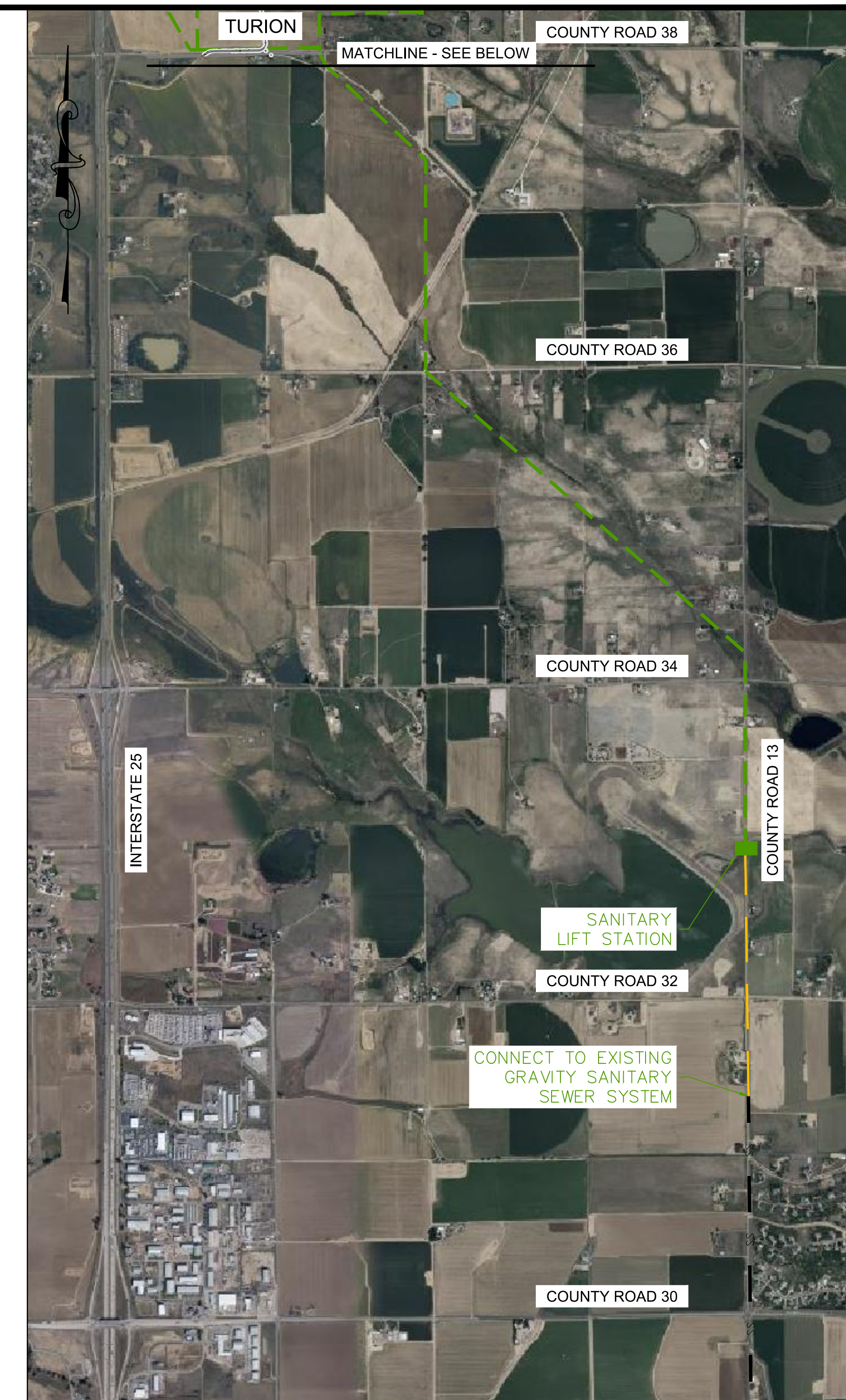
OFFSITE SANITARY SEWER OUTFALL SCALE: 1"=1500'
